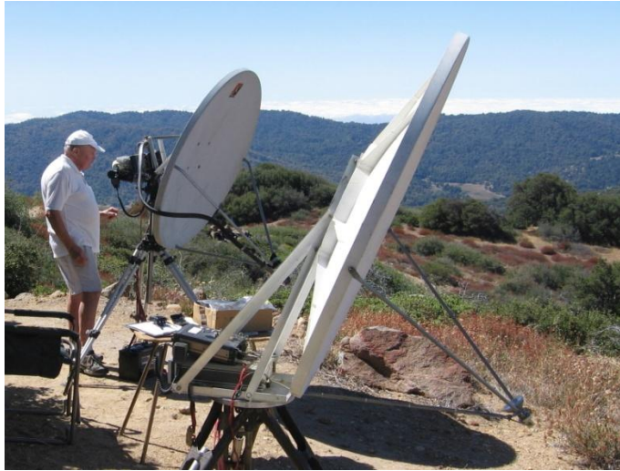
Jerry, K6DYD, operating on High Point near San Diego. He was joined by Dave, WB6TFC. They successfully worked far up the state into north-central California. Their stations are some of the strongest in the region running 25 watts into 4-foot dishes. (Photo WB6TFC)
