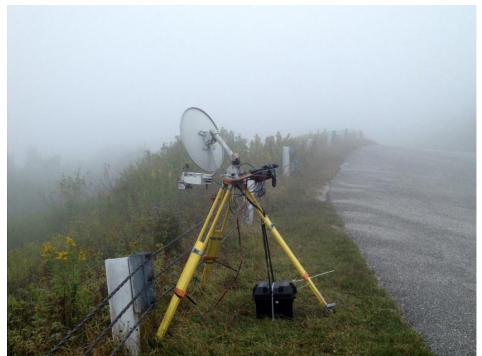
Tommy, W1AUV, spent Saturday morning of the September weekend on Mt Equinox. Notice the dish is tied using nylon ties to both the guardrail cables and the battery. Without those measures, the dish would have flown off the mountain. Although microwavers love the great horizons on mountains, the weather can make it a tough time. At the time of this photo, the temperature was 48 degrees and winds were about 30-40 mph. (Photo W1AUV)
