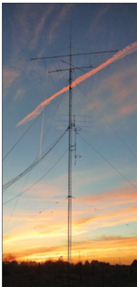
Hector, XE2K, used this eight-element Loop-Fed Array on 6 meters. [Hector Garcia, XE2K, photo]
