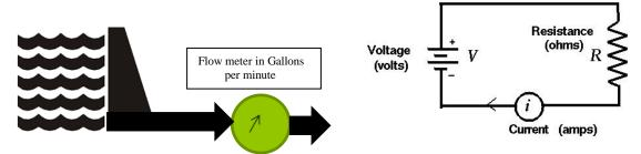
If we know the voltage and the resistance we can calculate the current that would be flowing in amperes using the following expression:
