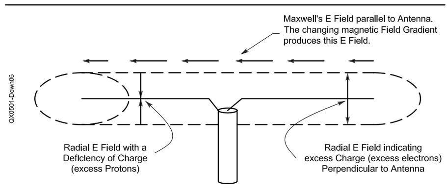
Fig 6—A dipole antenna and surrounding fields.
