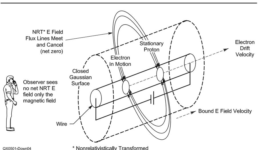
Fig 4—Electron motion in a wire and particle E fields.
