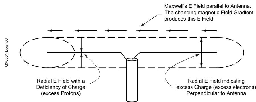
Fig 6—A dipole antenna and surrounding fields.
