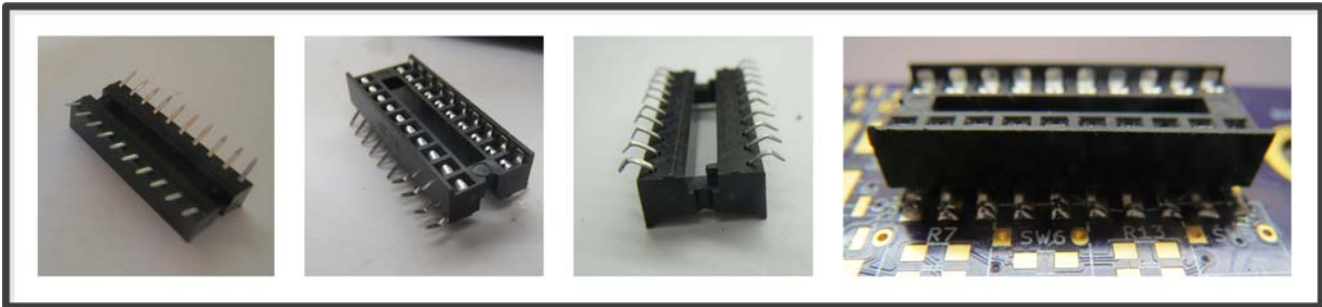
Figure 9 -- Converting 20-pin DIP through-hole socket to 20-pin DIP SMD Socket
