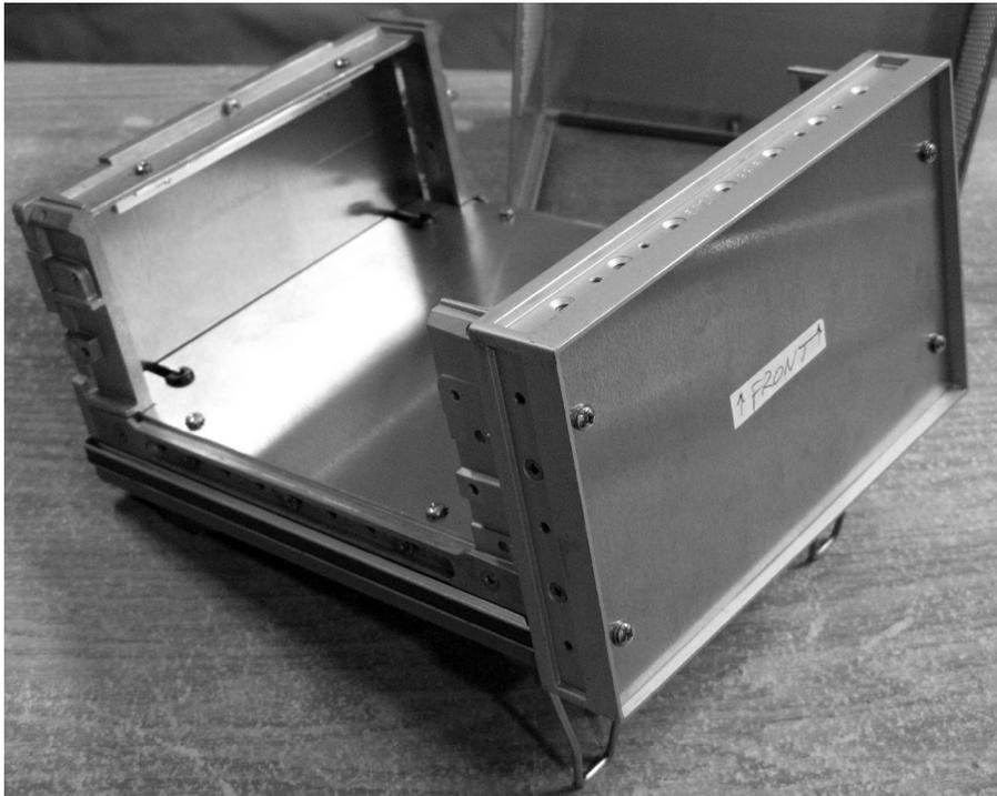
Figure 4 — Finished enclosure showing sheet aluminum panels installed.
