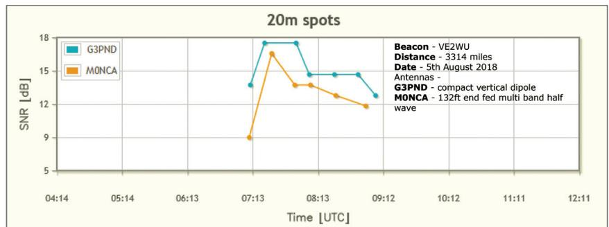
Figure 6 — An antenna comparison on August 5, 2018.
