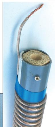
▼ Figure 4 — The copper pipe installed.
