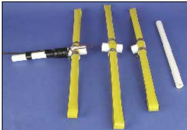
Figure 5 — Disassembled beam ready for transport.
