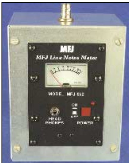
Figure 6 — Shielded MFJ-852 mounted in metal Bud box.
