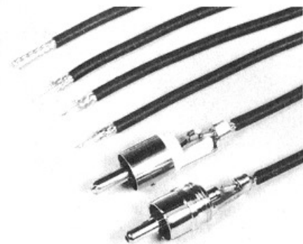
Fig 5—Installing a phono plug to coaxial cable is easy: Bare enough cable braid to clear the connector strain relief; remove about half the braid; strip about 1/16 inch of insulation from the center conductor; tin the center conductor, braid, center-conductor contact and the inside of the strain relief; slip the connector shell, facing the right way, onto the cable; solder the cable center conductor to the plug's center-conductor contact; crimp the strain relief around the braid and solder it; and install the shell. This photo shows unshielded and shielded (lowermost) phono plugs installed on RG-174 coaxial cable. Although the shielded plug allows you to continue the cable center conductor through to its center-conductor-pin tip, doing so offers no advantage and merely uses more cable.
