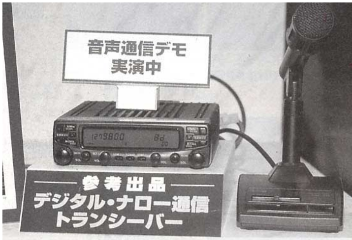
Photo showing the 1.2 GHz digital transceiver that operates at a low speed audio of 2.4kbps.
