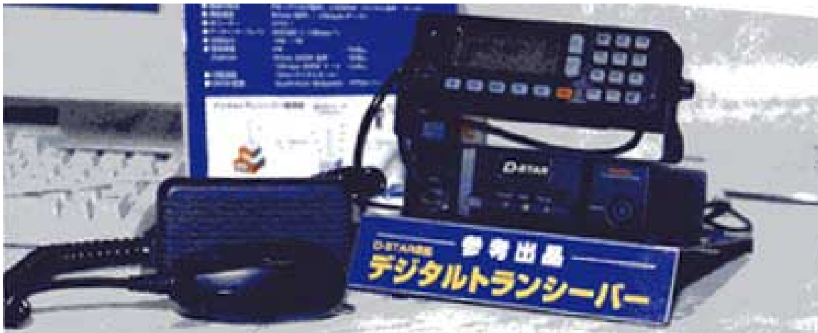
Photo 1: 1.2 GHz digital transceiver. Photo shows 8kpbs voice communication demo.
